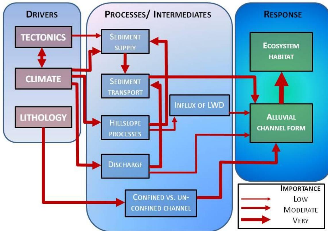
**Figure 4.4.** Conceptual model outlining the drivers, intermediates and processes, and outcomes behind river morphology in a sediment-dominated system such as the CCR. See text for details.
