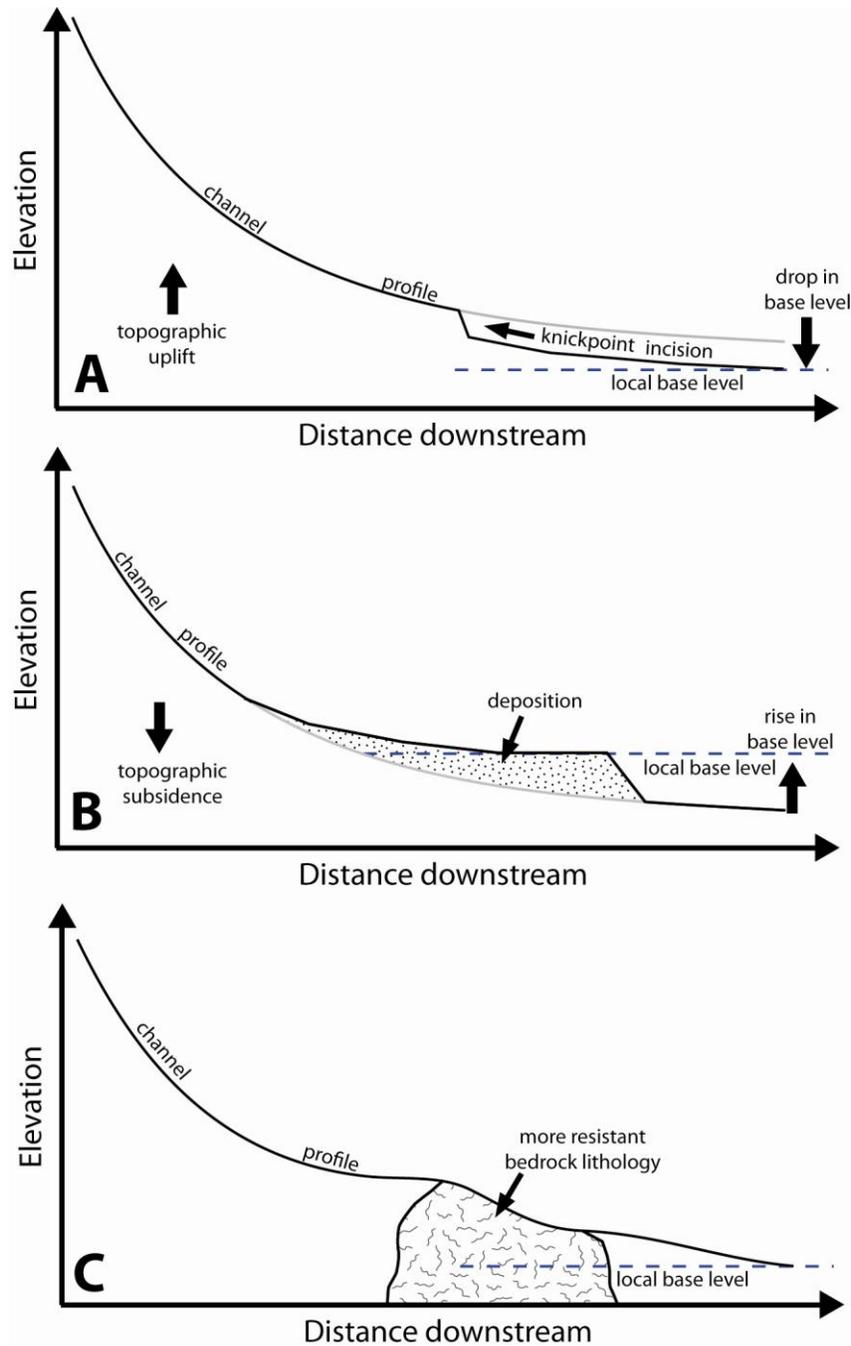
**Figure 4.2.** Perturbations to the longitudinal profile of a stream channel. **(A)** Relative drop in base level via tectonic uplift of the catchment or local base level fall. **(B)** Relative rise in base level via tectonic subsidence of the catchment or local base level rise. **(C)** Variations in downstream lithology. See text for details.
