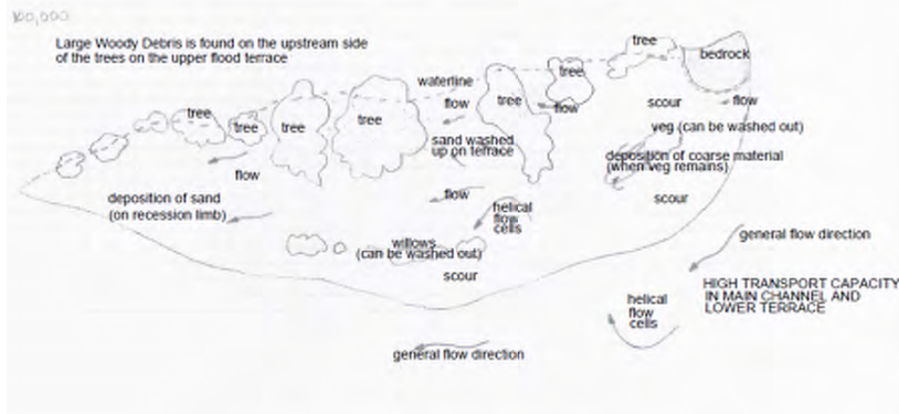
Figure 3.11 – Flow and waterline at Indian Bar during 100-year flood event.
